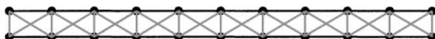
FIG. 10. Two strings of immersed boundary points and a set of elastic springs form a plate.
