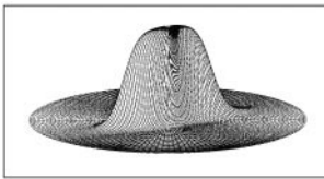
FIG. 2. Solutions of f_t + \frac{r}{2} \sin 2\theta f_r - \sin^2 \theta f_\theta = 0 at selected times. Parts (a), (b), and (c) are numerical solutions with \Delta\theta = \frac{\pi}{N} , N = 16, 32, 64 , respectively; (d) is the true solution.
